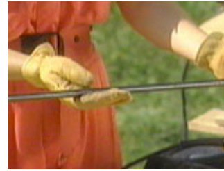
The axle is a steel rod available in a hardware store
