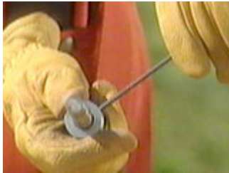
Slide on a bushing and secure it in place with the set screw
