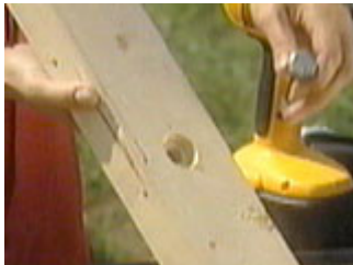
Drill a one inch diameter hole half an inch deep followed by a half inch hole through the board
