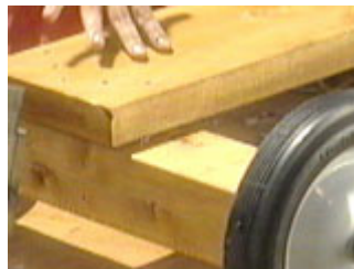
Attach the rear axle unit to the chassis with screws
