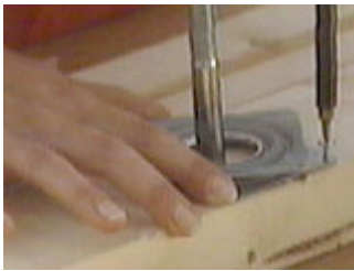
The 'lazy susan' hardware is centred on the bolt and attached with screws
